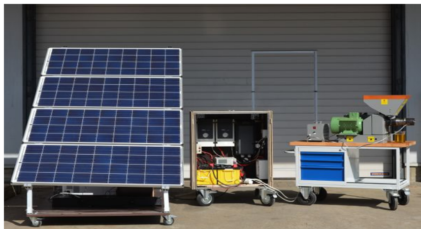
Fig. 8 Sesame oil extraction solar energy system designed by the University of Hohenheim
