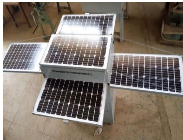
Fig. 5 Foldable and mobile onsite power supply for rural communities designed by the Federal Polytechnic Nasarawa
